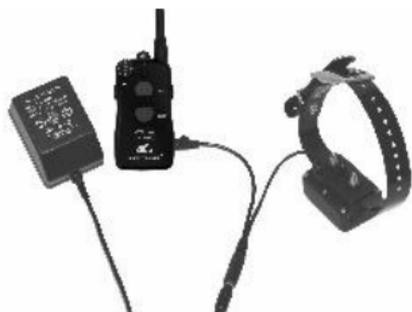
2. Plug the charger into a standard electrical outlet.
